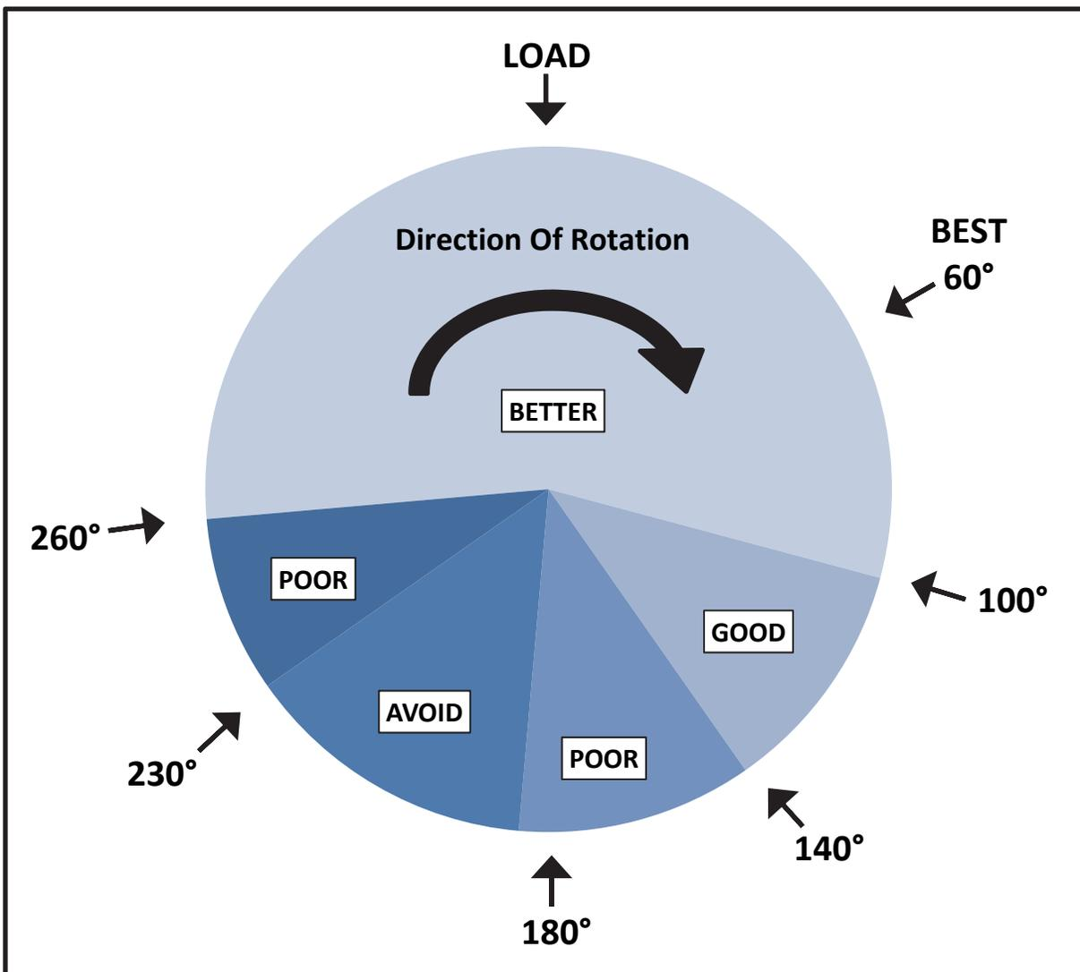
(The illustration shows the optimum engine oil feed hole location for a camshaft that is turning clockwise as viewed from the front of the engine.)
